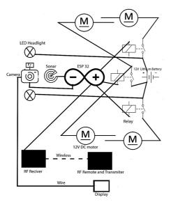
Figure 2. Circuit Diagram of the Under Water ROV (The symbol M indicates the motors used)
