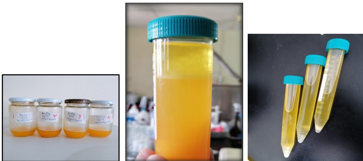
Figure 1. (a: The extraction mixture containing macerated pulp and organic solvents in 1:10 (dw:v) ratio b: The extraction mixture after being centrifuged c: Pigment oil
